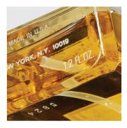
Ideal overt codes are permanent to prevent removal by unauthorized parties. Laser marking systems can provide high quality permanent codes on many package types.
